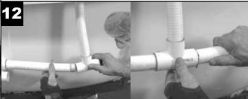
Glue one of the 11.5" hoses to the left side of the T-Connector and to the left side of the air coupling on the jet body. Repeat the process for the right side.
