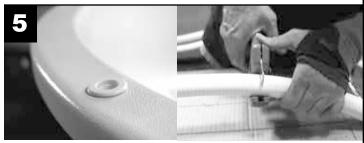
Remove air control knob from top flange of Cozy Cove. (Model HS604 is on the front left of the unit.) Then cut two (2) pieces of PVC hose (H02516) to 52" each.
