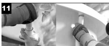
Cut five (5) pieces of hose to 11.5" and PVC cement it to the center hole of the 1" T-Connector (H00240) and the other end into the bottom of the Air Control Assembly (H00706) located under the top flange.
